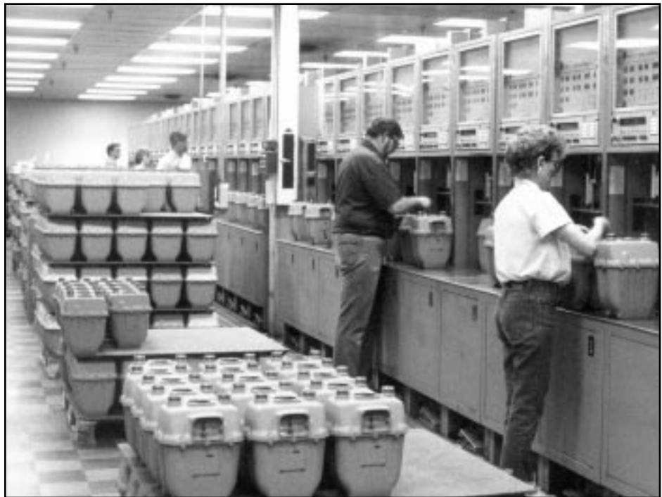
This is the residential gas meter proving room. In this room meters are individually calibrated to insure accuracy is within the tolerance demanded by you.
