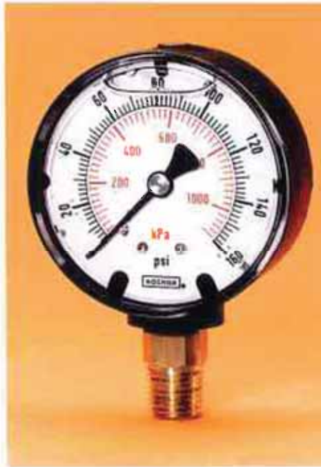
25.900 2½ INCH ABS CASE GLYCERINE FILLED ¼" NPT BOTTOM CONNECTION
