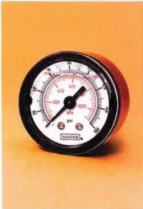
15.910 1½ INCH ABS CASE GLYCERINE FILLED ¼" NPT CENTER BACK CONNECTION
