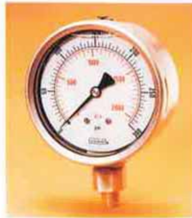
25.901 2 1/2 INCH STAINLESS STEEL CASE GLYCERINE FILLED 1/4" NPT BOTTOM CONNECTION
